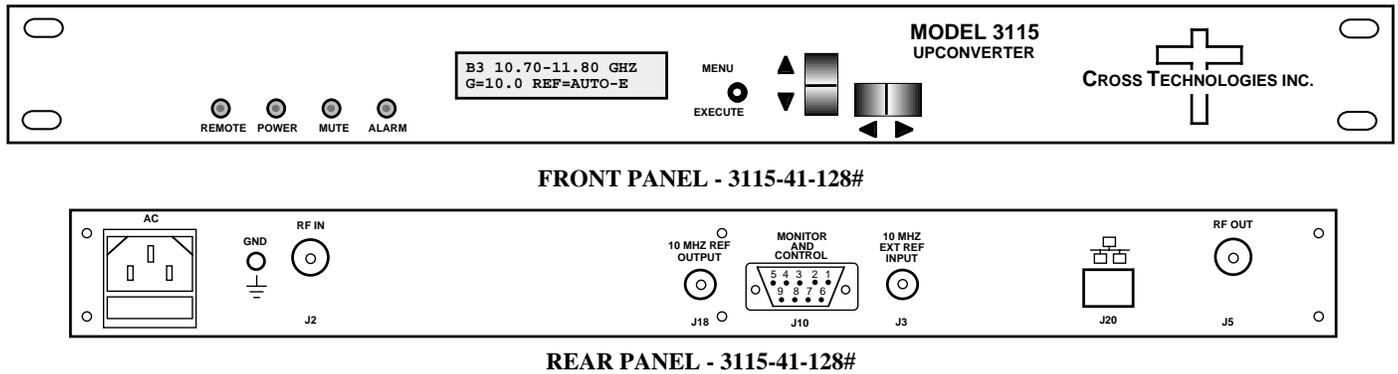
**FIGURE 1.1 3115-41-128# Front and Rear Panels**
