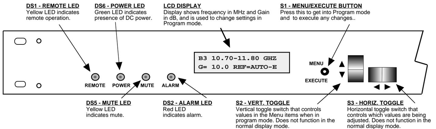
FIGURE 2.2 3115-41-128# Front Panel Controls and Indicators
